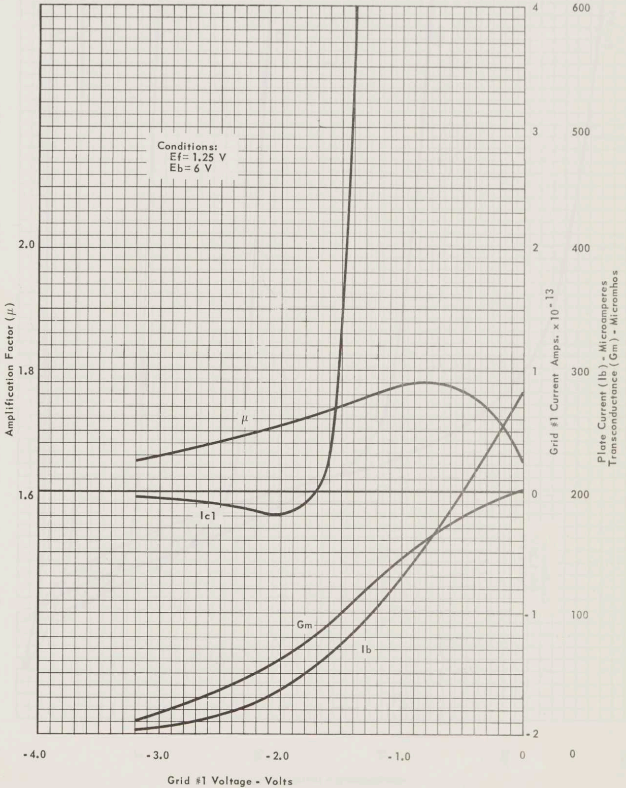
AVERAGE TRANSFER CHARACTERISTICS (Triode Connected)
